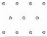
Grid pattern of injection sites, typical of curtain or bladder injection. Two feet on center
