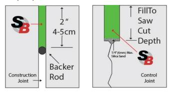
Joint Preparation: Thoroughly remove all dust, debris and moisture from joints to not compromise adhesion. Use a dustless concrete saw with diamond blade. For clean concrete surfaces, primer is not needed. Caution: Thoroughly read SDS and installation instructions prior to opening containers or dispensing.
