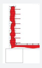
Schematic view of the gel's effect in brickwork. The injection gel is distributed between bricks, joints, cavities and cracks through the drill-holes. The bottom drill-holes level acts as a water stop against capillary rising dampness.
