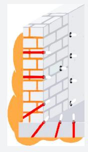
Schematic view of the working principle of SealBoss 2400 SealGel. The gel is injected from the inside of the structure via drill holes.
